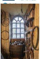
4. A cooper made barrels for storing wet and dry goods for shipping around the world. This trade required tools such as an adze, a croze, a drawknife, a froe, and a cresset to shape wooden staves (narrow lengths of wood) held together with wooden or iron hoops. What tool are the drawknives, froe, and froe maul sitting on?
